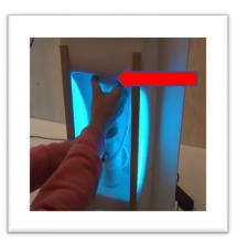
To turn on the Vitality Booth turn the timing knob to the desired time. Time can be set up to 30 minutes.
