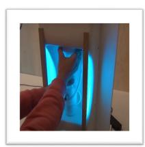
Unthread the turbo mill off the bottom and brush off any salt left on the turbo mill.
