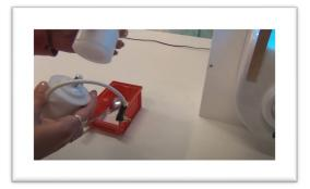
Brush out the inside of the air channel piece.
