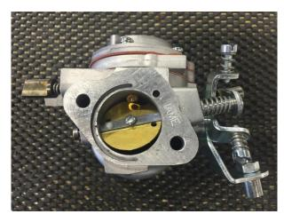
Picture above shows butterfly without "dimples", and shows butterfly in slightly open position if not tightened properly.
