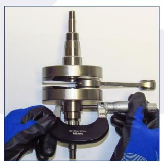
The crankshaft and the micrometer have to be at the same ambient temperature.
