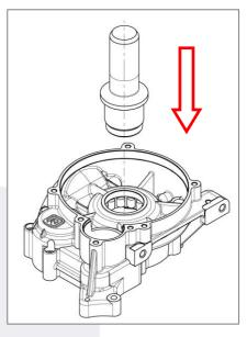
To remove the inner ring from the crankshaft, use the specific puller (IAME ATT-048X). The lip grabbing the spacer is necessarily thin, be careful to fit it exactly on the crankshaft. Tighten the 2 Allen screws M8x30, then tighten the M12 screw (Hex.19) until the complete extraction of the inner ring, blocking the puller body.
