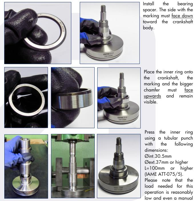
rack press is sufficient. The tube-punch helps to press the inner hole parallel to the crankshaft axis.
