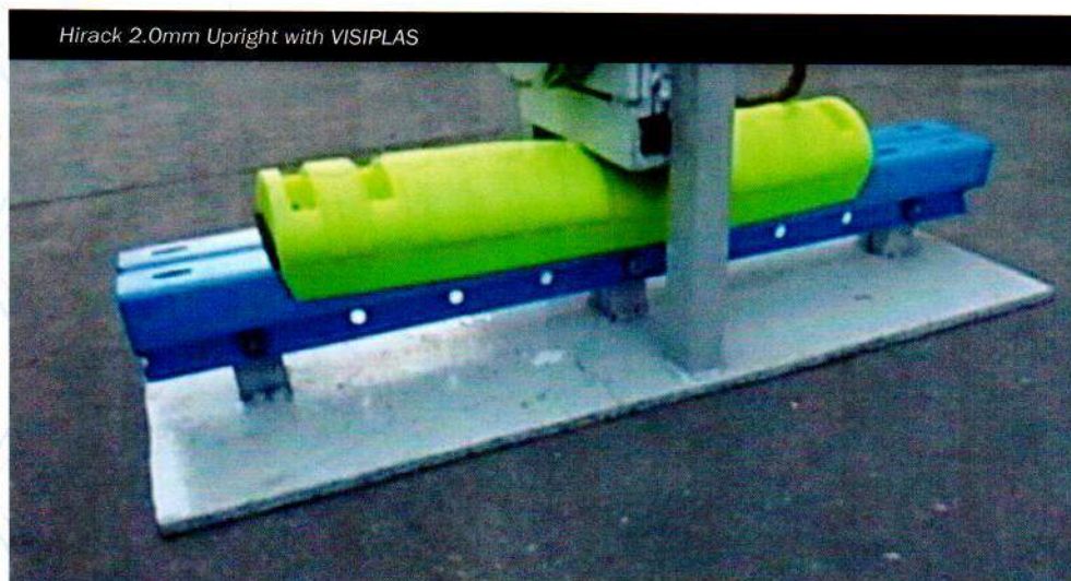
This photo shows the VISIPLAS during the impact. Note the deflection of the VISIPLAS as the impact force is absorbed.
