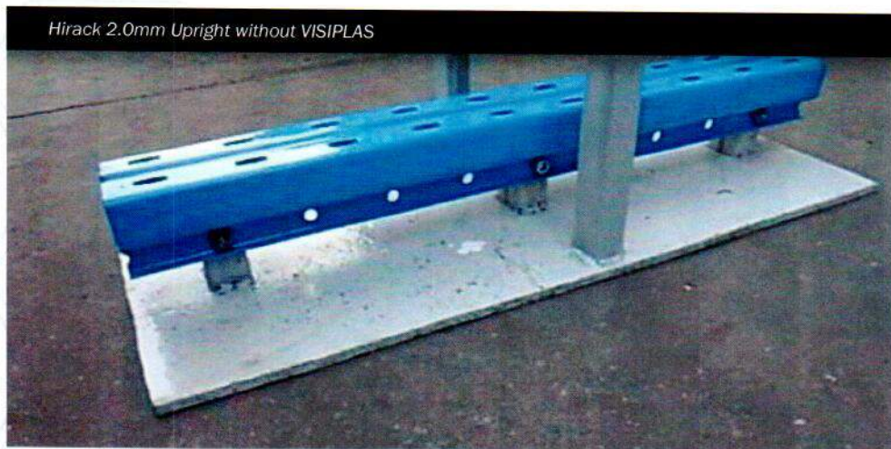
This photo shows the upright without VISIPLAS prior to impact.
