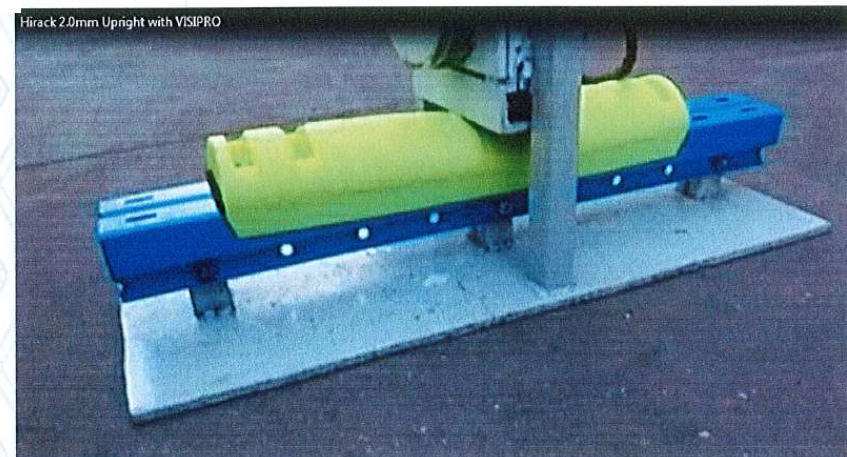
This photo shows the VISIPRO during the impact. Note the deflection of the VISIPRO as the impact force is absorbed.
