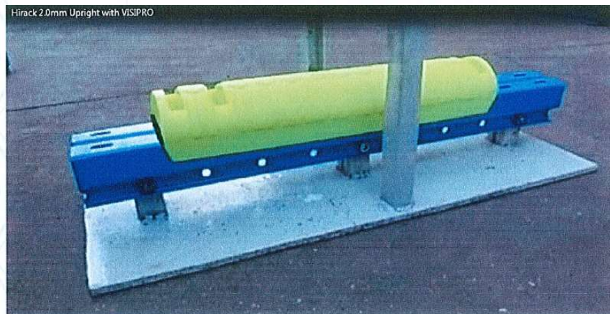
This photo shows the VISIPRO fitted to upright prior to impact.
