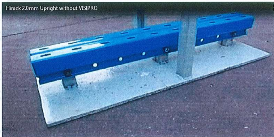
This photo shows the upright without VISIPRO prior to impact.
