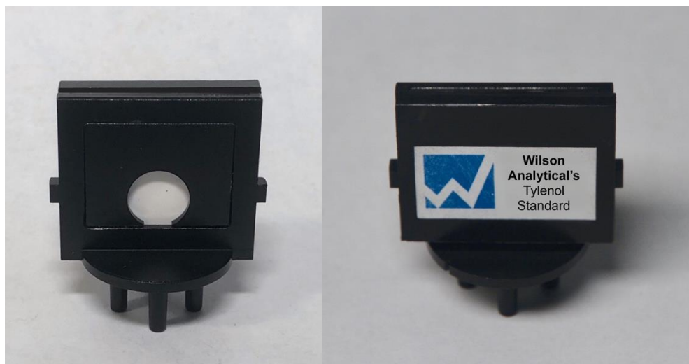
Figure 17. Tylenol Pellet Reference Standard for checking the Raman One and ensuring that the fine adjustment dial is centred.
