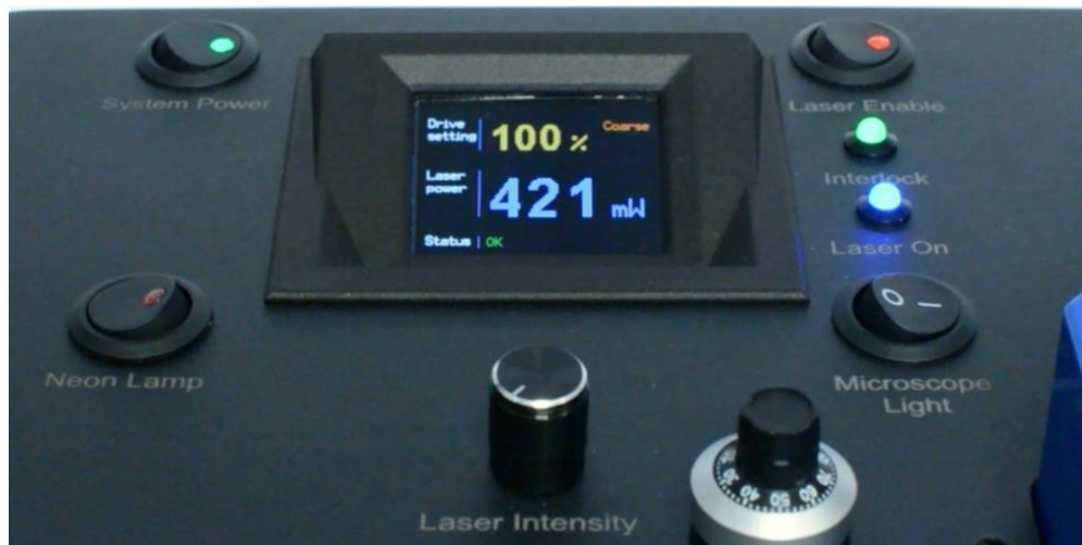
Figure 5. Image of the Laser Display Screen which indicates 100% Drive setting and 421 mW Laser power. The Interlock is satisfied, and the laser is on as indicated by the indicator LEDs.
