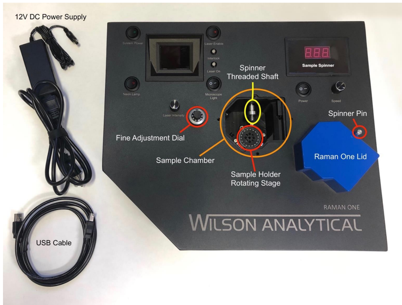
Figure 1. Raman One parts identification. Sampling accessories are sold separately.
