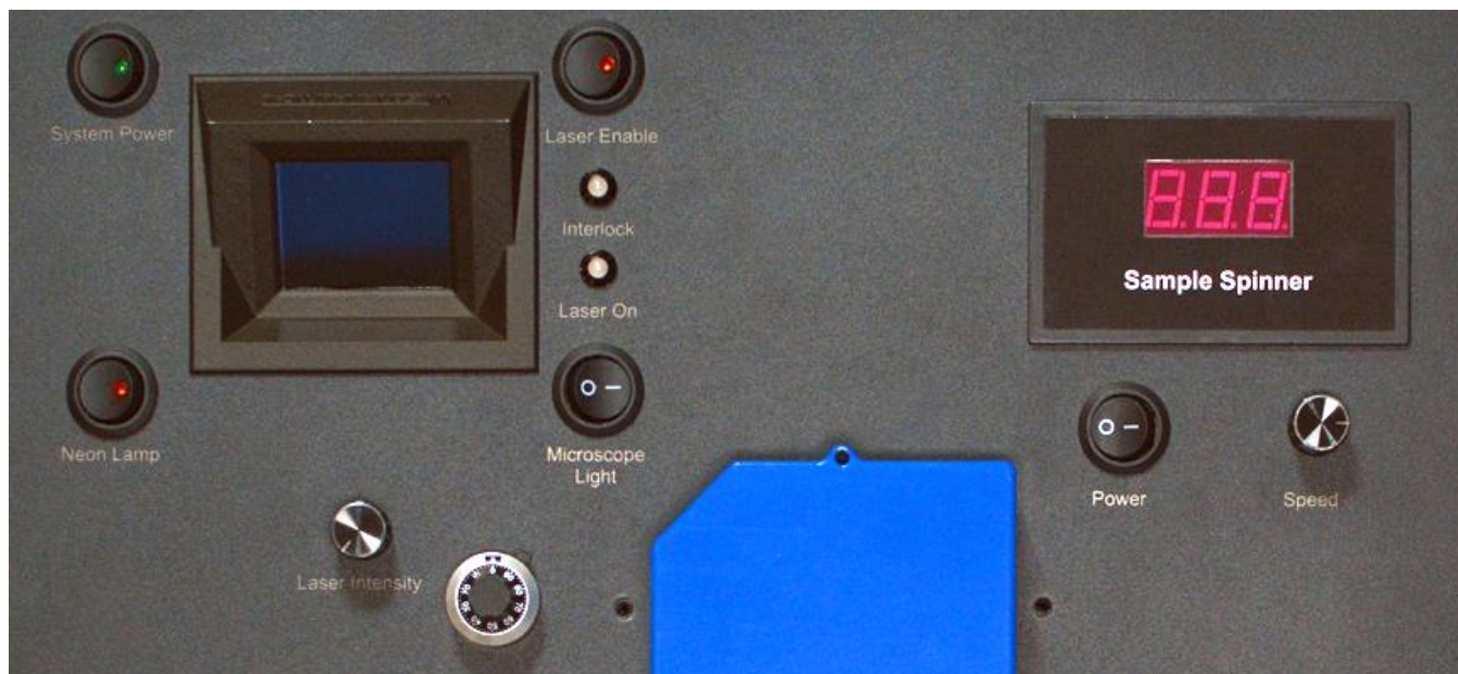
Figure 6. Image of the top of the Raman One, showing the power switches, the LED indicators, and the sample lid on the top of the unit (which covers the sample spinner and the sample holder rotating stage).
