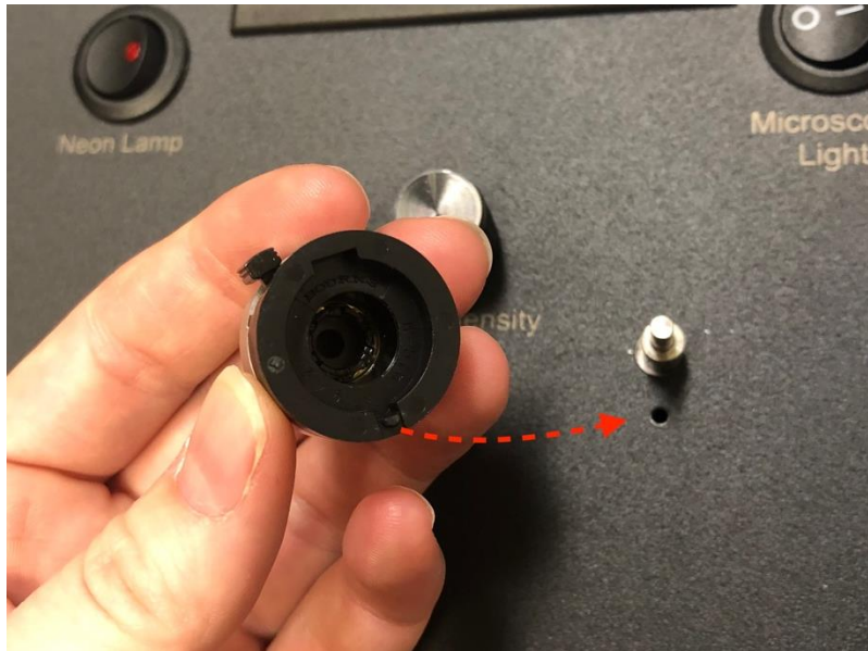
Figure 21. Align the small pin on the bottom of the fine adjustment dial to the small hole on the Raman One case.
