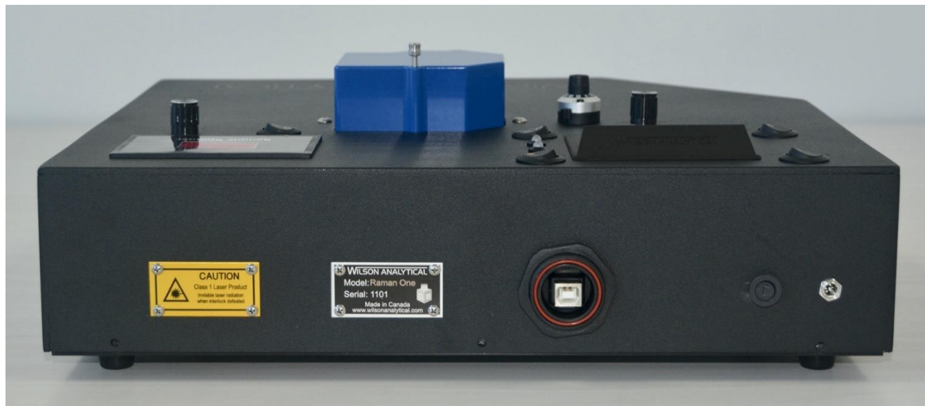
Figure 4. Image of the back of the Raman One showing (from left to right): the Laser Caution label, the Wilson Analytical tag, the USB data port, the 5 A Fuse, and the 12 V power port.
