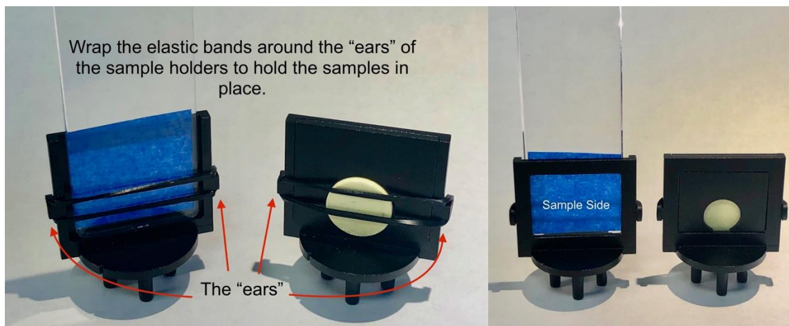
Figure 13. Left: sample holders with elastic bands wrapped around the backs of the samples to keep them in place. Right: the front view of the samples in the sample holders. Note, the sample is placed on one end of the slide represented by the blue tape in the photograph.
