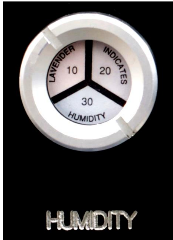
Figure 18. Humidity indicator located at the back of the QuatBox™
