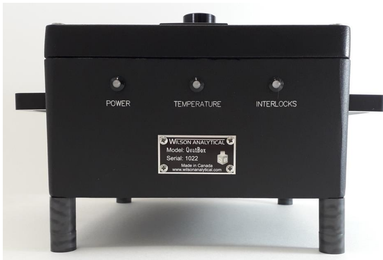
Figure 10. LED indicators at the front of the QuatBox
