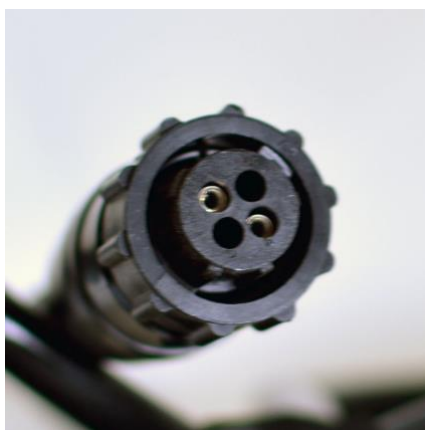
Figure 8. DIN power plug on the QuatBox end of the power cables. This DIN plug makes a waterproof seal with the DIN power socket on the back of the QuatBox and has a rotating locking collar to securely hold the cable in place.
