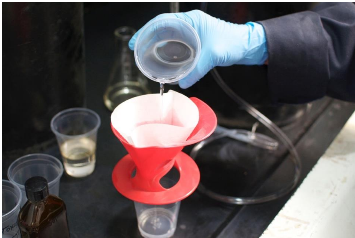
Figure 19. Filtrating a Sample using a #2 Coffee filter, before testing
