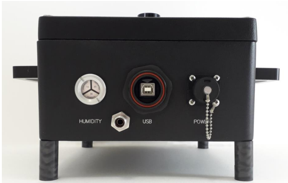
Figure 5. Connections on the rear of the QuatBox. Note the cap in place over the power socket.
