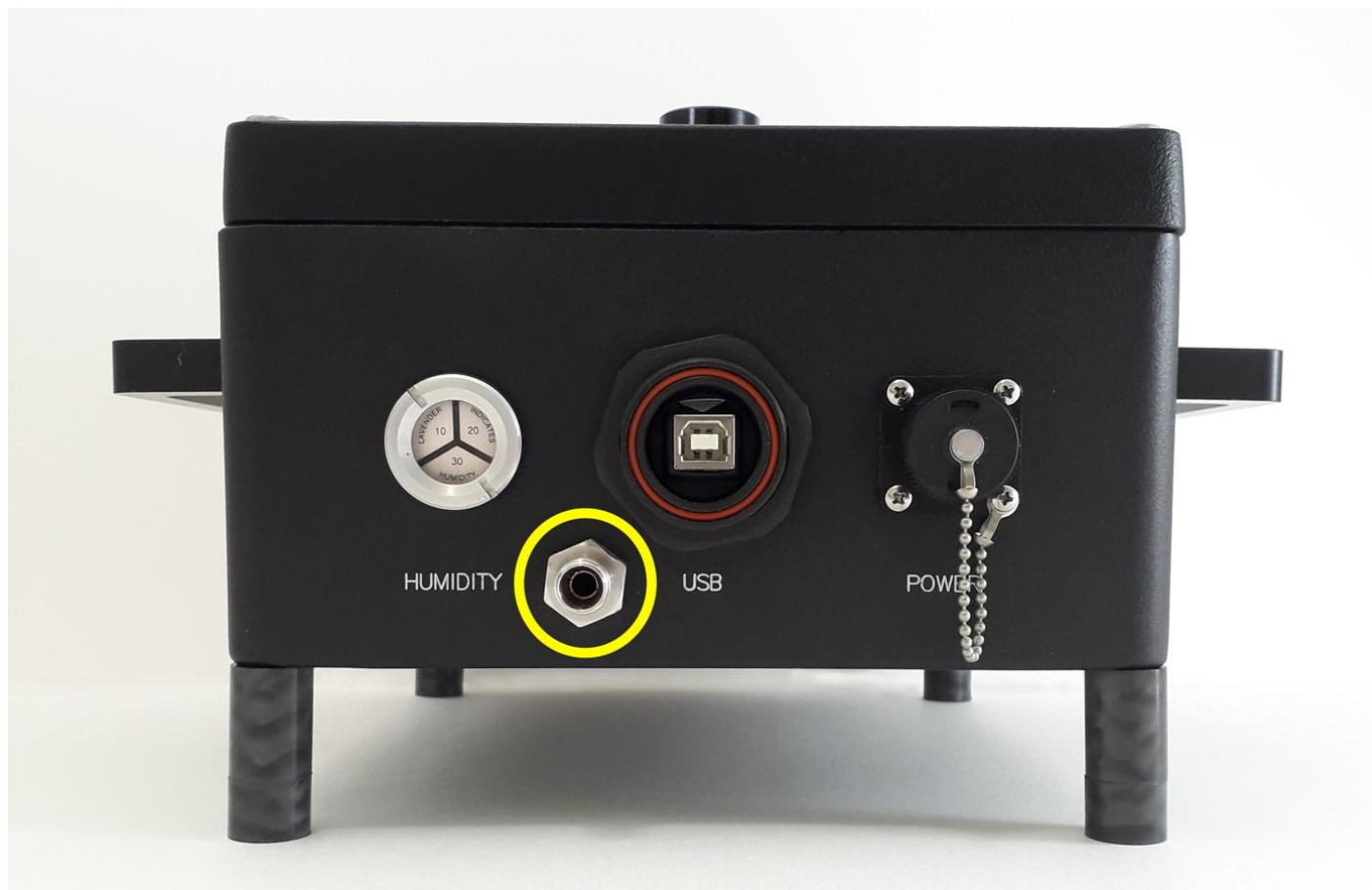
Figure 15. The stainless-steel drain fitting on the rear of the QuatBox™, circled in yellow.
