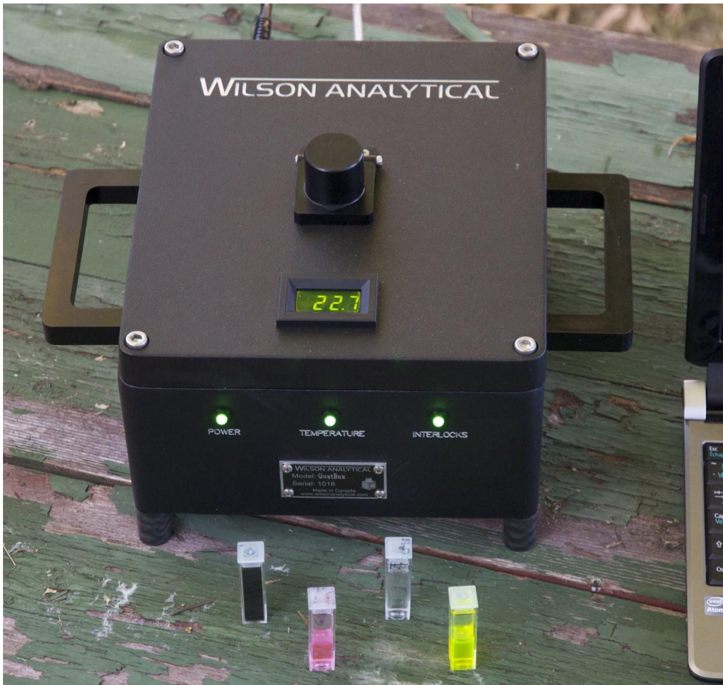
Figure 11. The QuatBox™ with all three of the LED indicators showing green, indicating the instrument is ready for testing. Note the sample temperature display on the top of the unit.
