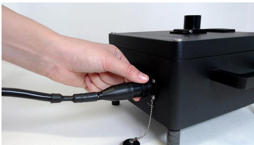
Figure 9. Connecting and locking the DIN power plug to the rear QuatBox power socket.
