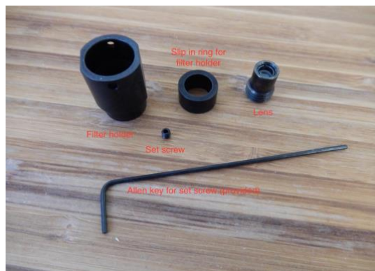
Figure 9. Expanded view showing spectrometer filter holder parts and a lens.
