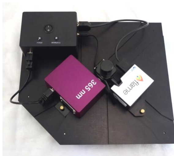
Figure 2. Overview of the OPS showing the cuvette holder positioning and the interlock cable connection to the control box. The 365 nm light source and the Flame spectrometer are mounted at a 90° angle.
