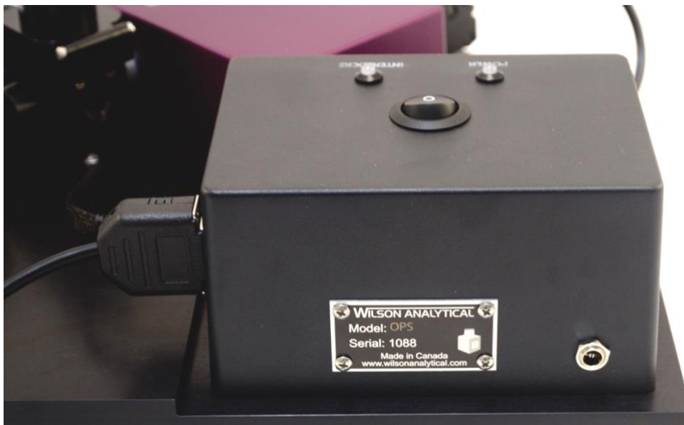
Figure 13. The back of the control box. Note the power switch and the LED indicator lights on the top, the DB9 connection on the side, and the power connection on the back.
