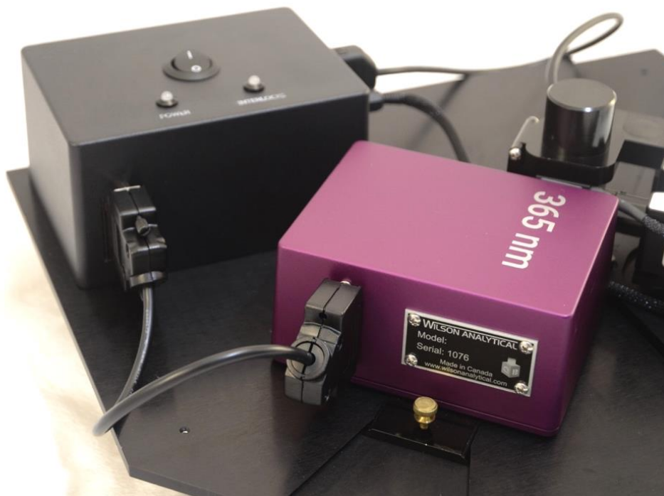
Figure 7. The cable connection between the control box (left) and the light source (right). Note that the thumbscrew on the light source slide faces the outside edge of the OPS base plate.
