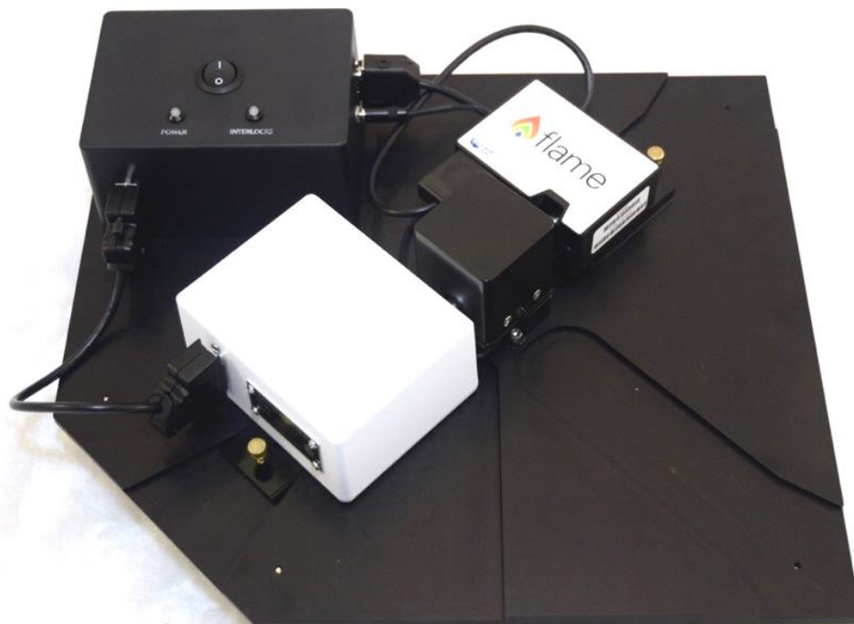
Figure 10. The solid sampler in absorbance mode. Note the 180° geometry between the light source and spectrometer.
