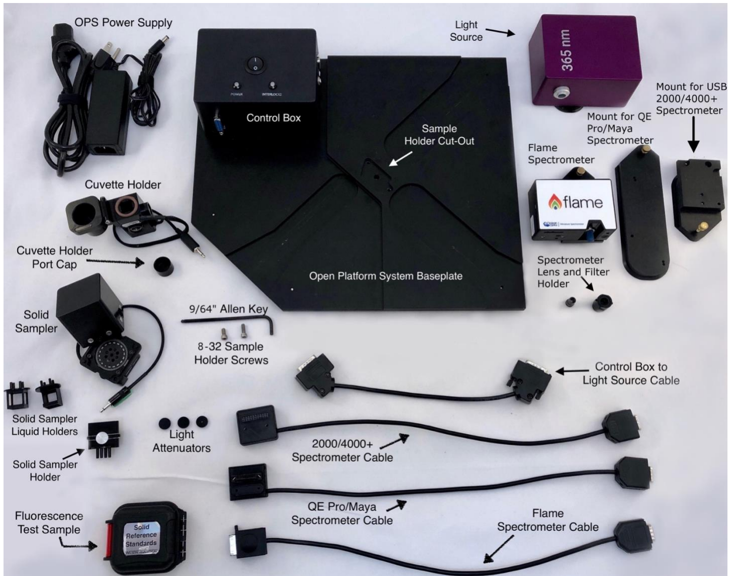
Figure 1. Open Platform parts identification (spectrometer and accessories are sold separately).
