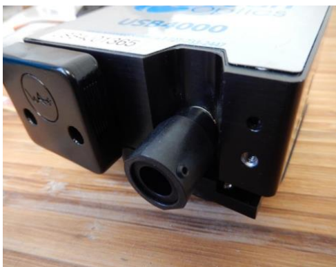
Figure 8. Filter holder and lens mounted on a USB4000 spectrometer.
