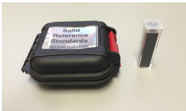
Figure 20. QC test sample for checking the fluorescence operation of the OPS at 365 nm.
