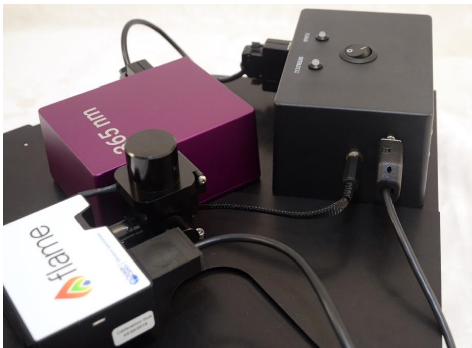
Figure 11. The cable connection from the spectrometer to the DB9 connector on the control box.
