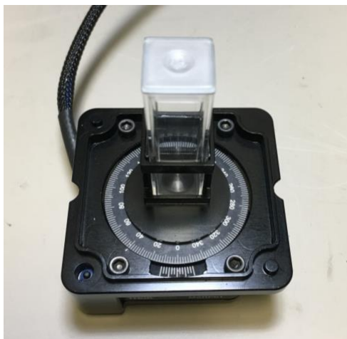
Figure 18. Offset cuvette holder (with cuvette) mounted on the rotation stage of the solid sampler base.
