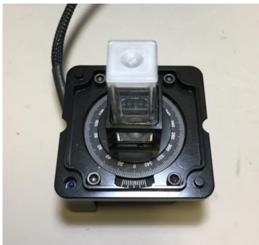
Figure 19. Centered cuvette holder (with cuvette) mounted on the rotation stage of the solid sampler base.
