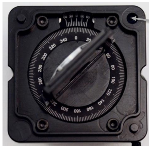
Figure 5. The location of the rubber pad (with the embedded interlock microswitch) in the base of the solid sampler.
