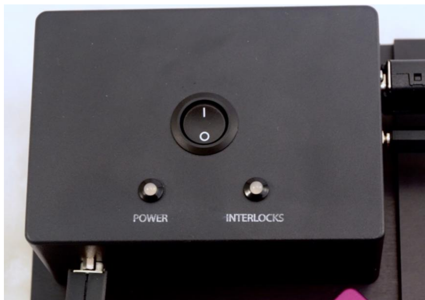
Figure 14. Power switch, Power LED, and Interlock LED. See Table 2 for LED Indicator colours under various spectrometer conditions.
