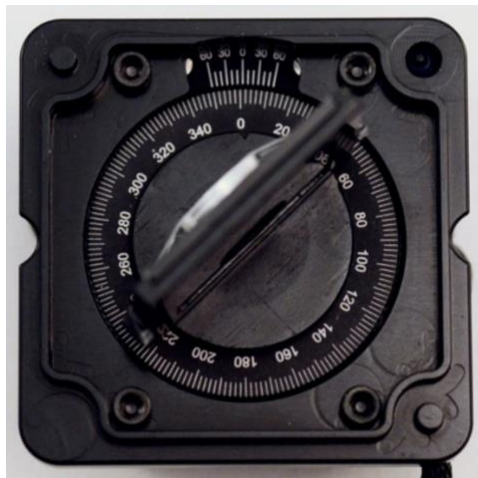
Figure 17. Lining up the solid sampler rotation stage to 0^\circ so that the sample mount sits at a 45^\circ angle to both the light source and the spectrometer.
