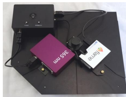
Open Platform-fluorescence configuration with 365 nm light source and Ocean Optics Flame Spectrometer.
