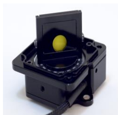
Solid Sampler with pressed pellet
