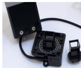
Solid Sampler with "centered" and "offset" cuvette holders
