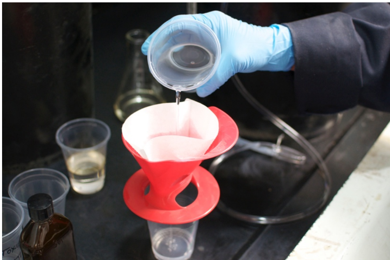
Figure 6. Sample being filtered prior to analysis on the LabBox
