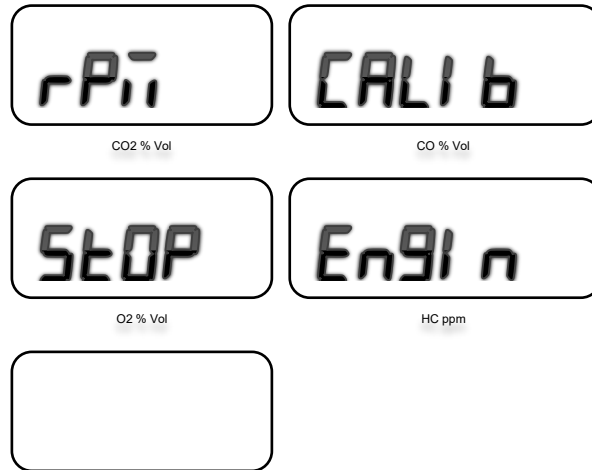
Figure 12 – RPM calibration screen, reads "RPM Calib, Stop Engine".
