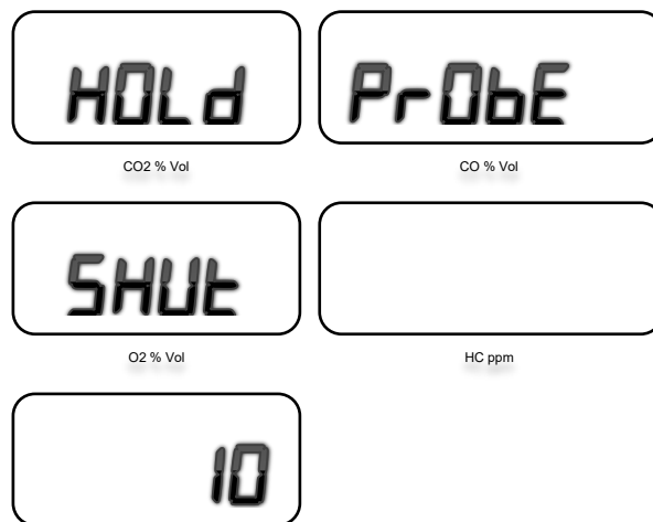
Figure 11 - Hold sampling probe shut for 10 sec.
