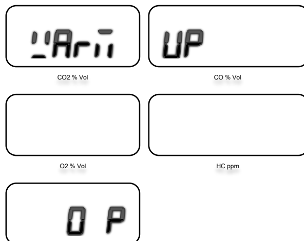
Figure 7 - Initial warm-up screen, reads "warm-up in progress 0%".
