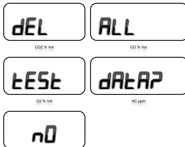
Figure 23 – “Del All Test Data?”, select Yes to clear the data or Cancel to go back.
