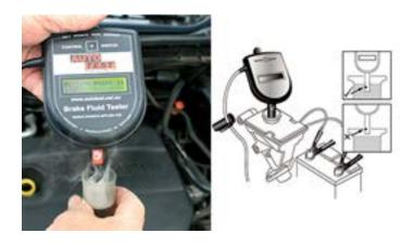
This user friendly tester helps to prevent vapour lock and corrosion of engine parts.
