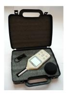
AutoTest Digital Sound Level Meter is used to measure and monitor noise levels to ensure that volume levels are within tolerances or an expected rage in any industrial or domestic application.
