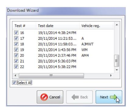
Select the tests that need to be downloaded and then press Next. Datalogger software will automatically download all selected tests.
