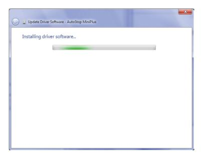
When Windows has completed installing the drivers for the USB interface, the following window will appear. Notice the COM port number displayed on the titlebar. The COM port will be used when downloading data from the meter using the datalogger software.
