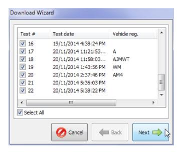
Select the tests that need to be downloaded and press Next. Datalogger software will then download the selected tests. While downloading, the LCD screen of Mini Plus will display "Uploading 00%...."
