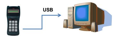
Once the USB cable is connected to the PC, switch ON the Brake Meter by pressing the ON/OFF key. When the Brake Meter is switched ON, the PC will recognise the Brake Meter device and will search for the USB drivers.
