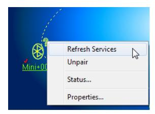
Once the pairing is established, refresh device services and connect using Bluetooth serial port service.
