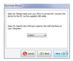
Select the COM port of the USB connection. The COM port is the same port obtained earlier during the USB drivers installation process. Make sure the brake meter switched ON and it is connected to the PC via the USB cable. Press Next to continue.
