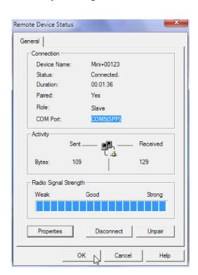
Once the Bluetooth connection is setup, the user can now download test results from Mini Plus using the Bluetooth interface. To download the results, open AutoStop Mini Plus datalogger software and click on "Download" button.
