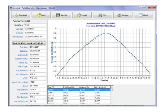
The menu buttons displayed on the top bar can be used to perform the following operations:
