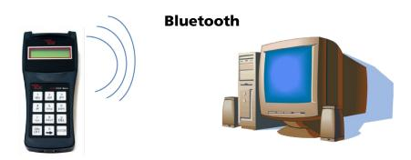
When connecting the Brake Meter for the first time using the Bluetooth interface, user will need to configure the Bluetooth connection. To configure the Bluetooth connection, open your Bluetooth manager program on your PC and search for Mini+#### device, where '#####' is the serial number of the brake meter.
