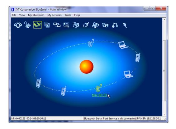
Select the device Mini+#### from the list of discovered Bluetooth devices and create pairing.
