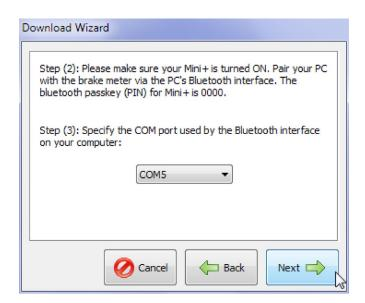
Make sure the brake meter is ON. Press Next to continue. Once the connection is established, the datalogger software will acquire a list of all tests currently stored on the device.
