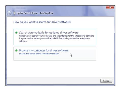
When the browse window is shown, select the USB driver folder located in the directory where the AutoStop Mini+ datalogger software is installed. On a 64-bit operating system, the default location where USB drivers are likely to be found is at "C:\Program Files (x86)\AutoTest\ AutoStop Mini+ Data Logger\USB Drivers". On a 32-bit system, the USB driver's folder would be at "C:\Program Files\AutoTest\AutoStop Mini+ Data Logger\USB Drivers".
