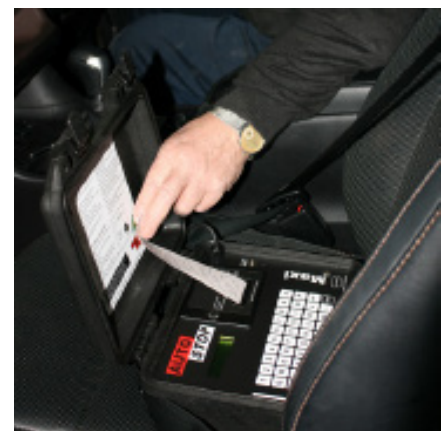
Figure 1: AutoStop brake meter in position ready for testing. Secure in position before turning on and starting any testing.
