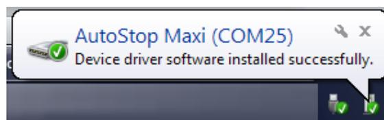
To verify the installation of the USB driver, locate “AutoStop Maxi/heavy” in the device manager under “Ports (COM & LPT)”. If the device drivers are successfully installed, there will be a COM port number written next to the device name. In the following example, the COM port number is “COM25”.
