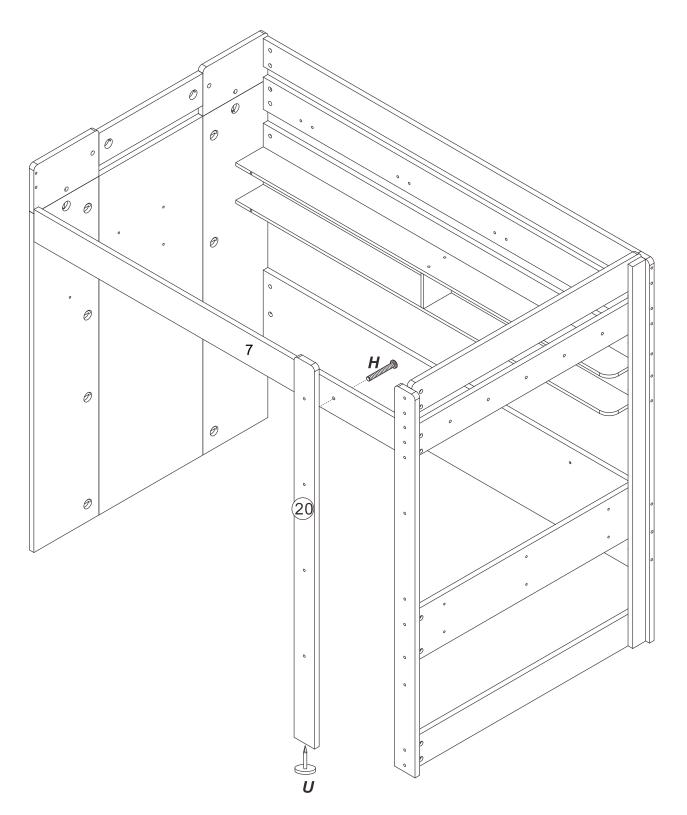
**Note:** on panel 7, the holes are not punched through so that the ladder side can be switched as needed, please use drill bit or the provided wood screw (R) to drill through to widen the holes.
