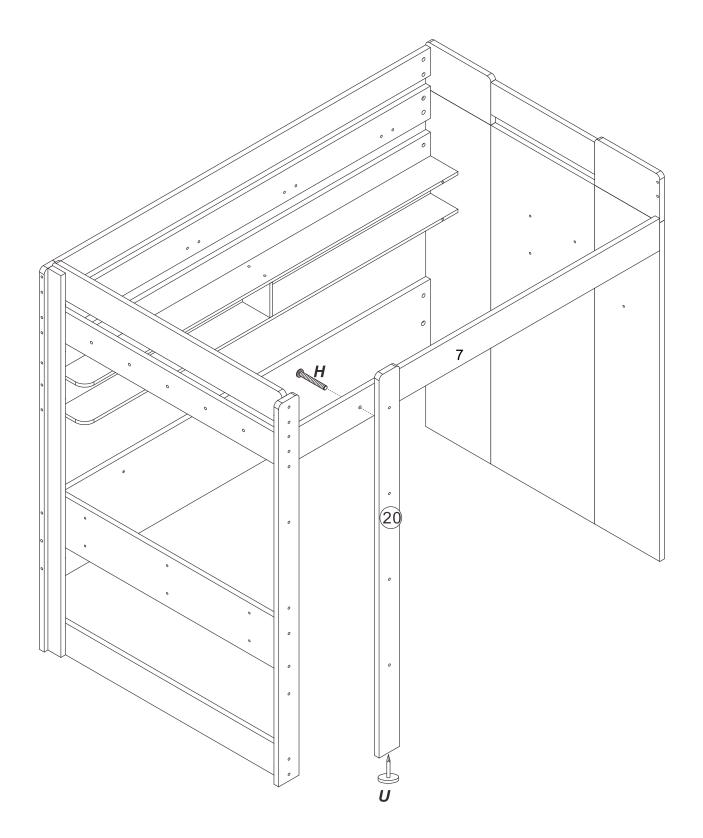
**Note:** on panel 7, the holes are not punched through so that the ladder side can be switched as needed, please use drill bit or the provided wood screw (R) to drill through to widen the holes.
