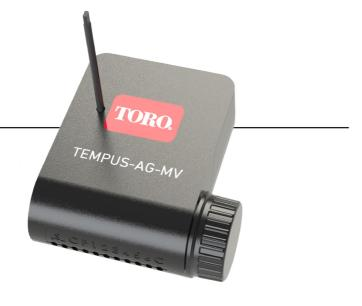
LoRa<sup>™</sup> controlled, battery-powered controller, IP68, to manage a Master Valve (or a pump control) equipped with an input for a rain or volumetric sensor.
