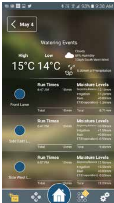
Result of Irrigation showing: Starting moisture level, irrigation, rain fall, evaporation equalling net moisture in root zone
