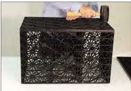
Place the large plate on top of the semi assembled module and fit into place. Use a rubber mallet to securely fit the pins into place.
