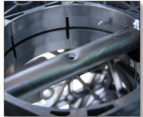
Punctured poly irrigation pipe
