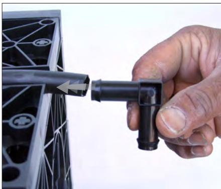
An end angle plug has to be inserted at the top module.
