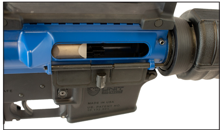
Figure 3-8 – Pulling the Charging Handle Rearward
