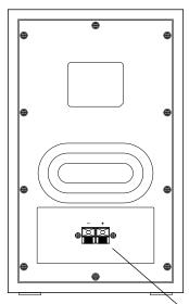
Push / Release, Spring-Loaded, Speaker In Jacks Connect to the optional, external Mondo Alto speaker.
