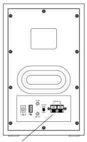
Push / Release, Spring-Loaded, Speaker Out Jacks Connect to the optional, external Mondo Alto speaker.
