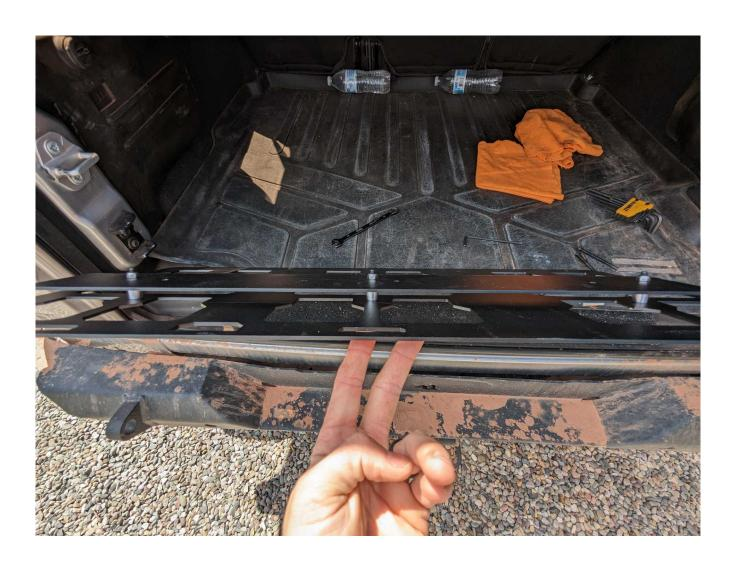
4. Using 3- M6 35mm bolts and 3- 3/4" spacers, loosely bolt the filler plate to the tailgate, starting with the center bolt, then the outer bolts. You will need to slip the 3/4" spacers behind the filler plate during this step.
