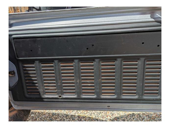
3. Using 3- M6 35mm bolts, 3- 3/4" spacers, and 3- M6 nyloc nuts, bolt the filler plate to the mounting panel. The Centerak Logo will be on the right hand side of the panel.
