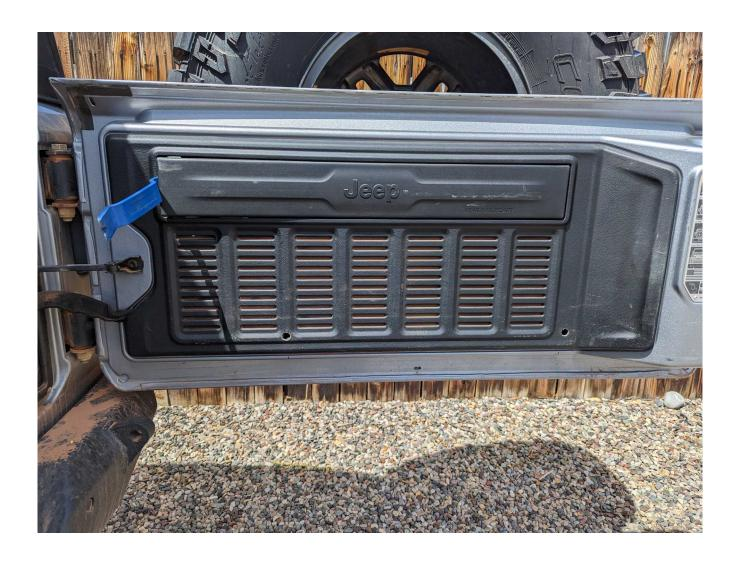
2. Orient Filler plate to line up with holes in tailgate. Note the orientation of all 6 holes.
