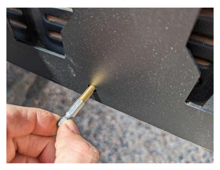
6. Remove the 3- bolts holding the filler plate to the tailgate. Using a 1/2" drill bit, drill out the factory tailgate panel where you marked it in the previous step. Then, install the 2- 2 3/8" spacers into the
