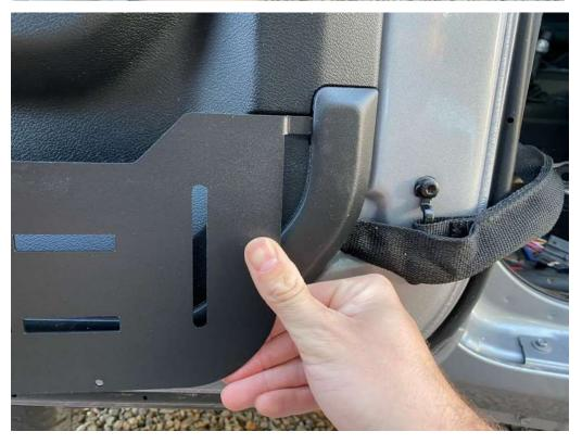
Once the front tab is in the hole slide the Mount forward.
