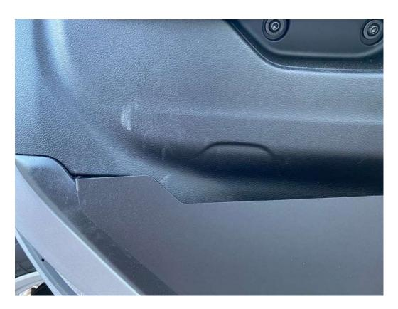
Now grab the Mount in the center and pull it away from the door while simultaneously pushing in on the panel near the front tab. The front tab will then be inserted into the hole where the door net elastic band was held in.
