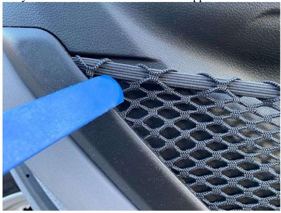
The elastic band must be slipped through the slot on in order to remove it.
