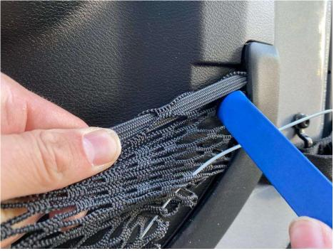
Once the front and rear of the elastic band have been removed from the door panel, grab the door net down low and firmly pull up to
