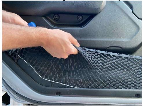
With the net now removed, use a T-20 bit to remove the 2 screws at the bottom of the door panel. These screws will not be re-used.
