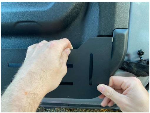
Now install the two provided spacers in between the Mount and the door panel. These go where the screws were removed from earlier in the installation.
