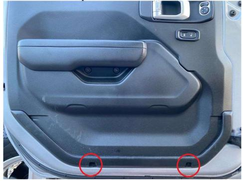
Insert the rearward side of the door panel mount into the hole that held the elastic band for the door net.
