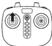
Move the left stick (throttle) fully up, after let it come back to the middle and the motors will start spinning.
