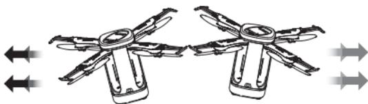
When the drone drifts to the left or right when it is hovering, hold the left joystick down and push the right joystick right/left until the drone stops drifting.
