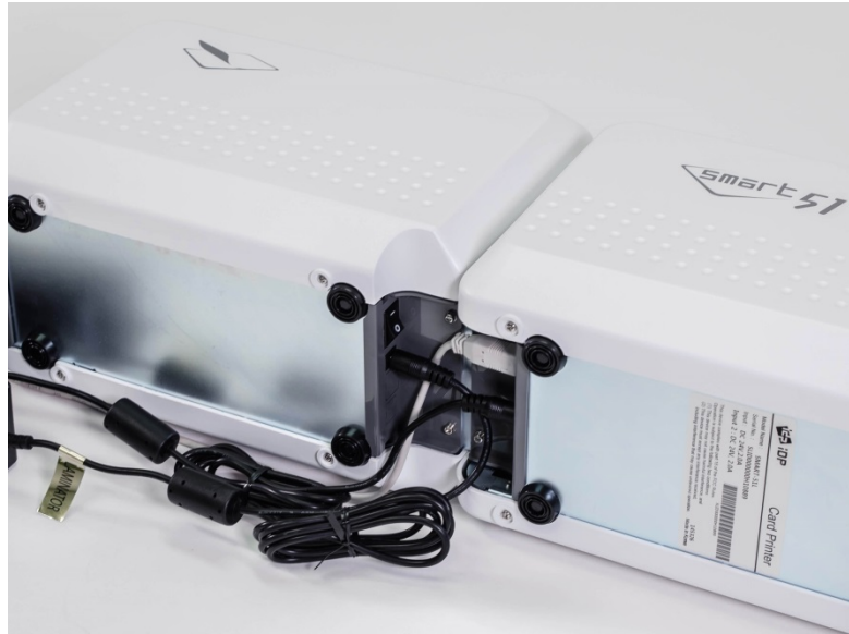
Figure 11 SMART-51L Connection of powers and USB cable - 1
