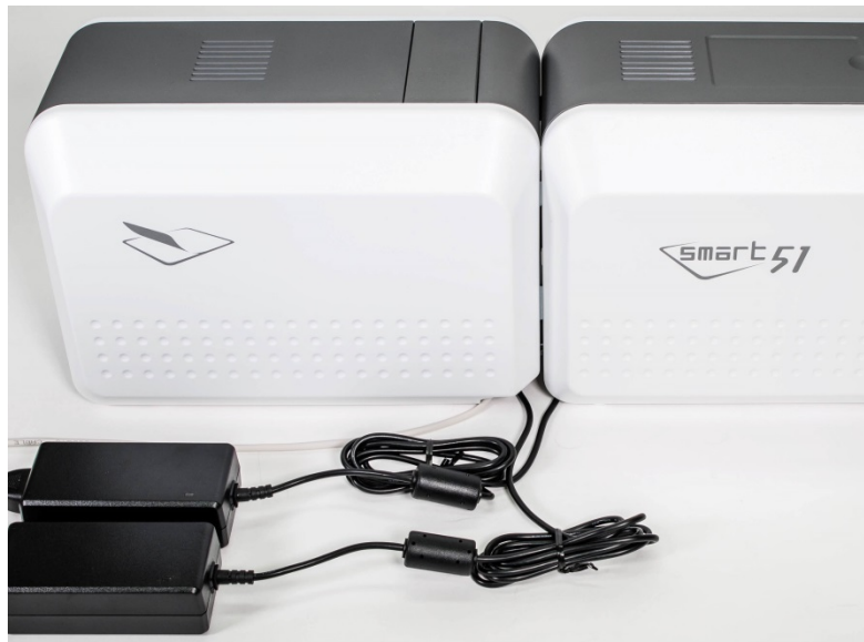
Figure 12 SMART-51L Connection of powers and USB cable - 2
