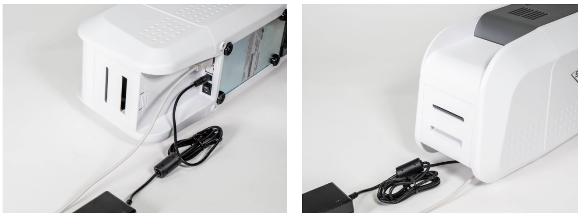
Figure 10 SMART-51D Connection of power and USB cable
