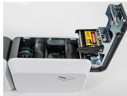
Figure 23 Installing the film cartridge
