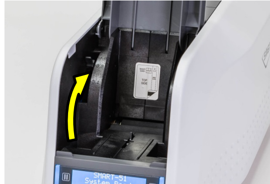
Figure 24 Adjusting the card thickness lever
