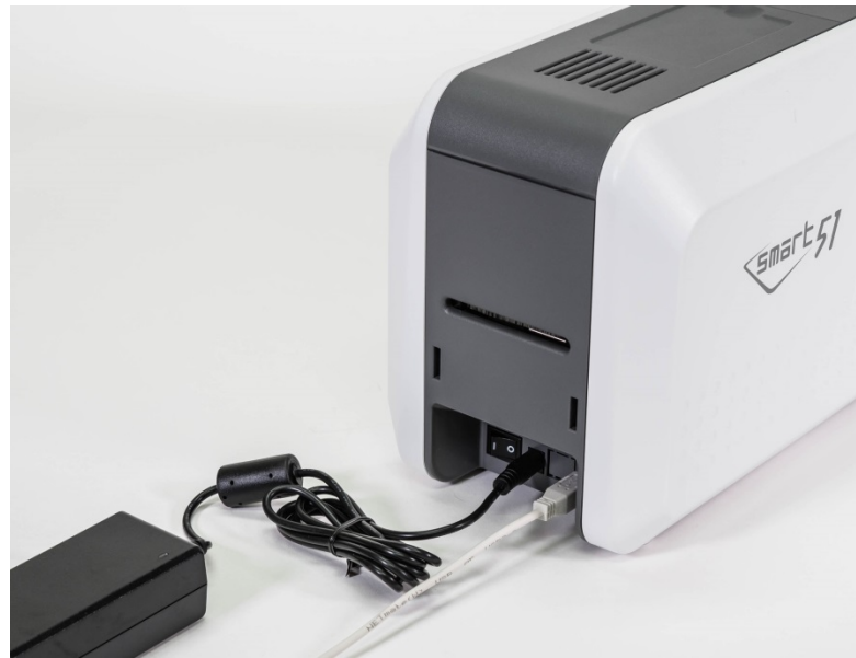
Figure 9 SMART-51S Connection of power and USB cable
