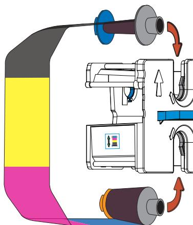
Load the print ribbon into the print ribbon cartridge until rolls click.
