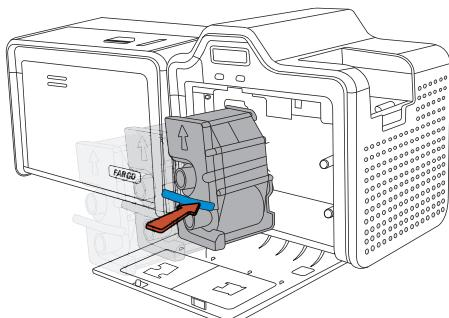
Insert the HDP Film cartridge into the printer until it clicks.
