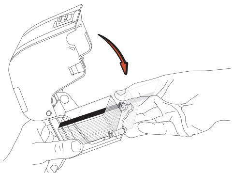
Load cards into the card input cartridge.
