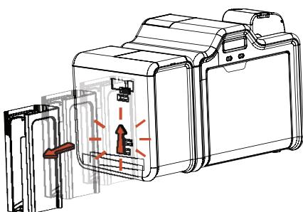
If applicable, remove card output hopper from the output side (left) of the printing module.
