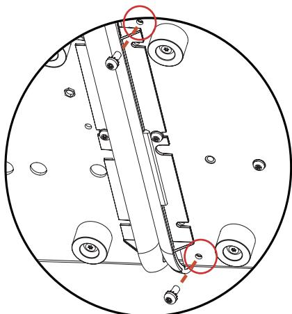
Using the tool and the 2 screws provided, secure the dual-sided printing module to the printer.
