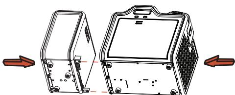
Slide the dual-sided printing module and printer together.
