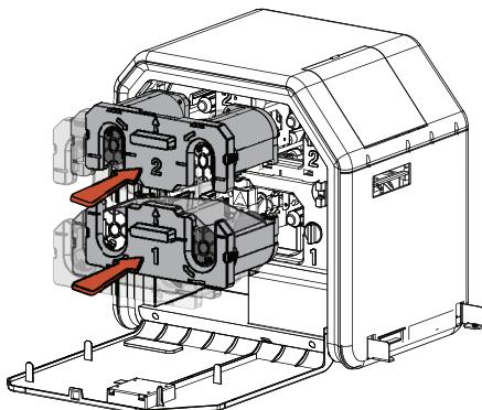
Insert the overlaminant cartridges into the lamination module until they click.
