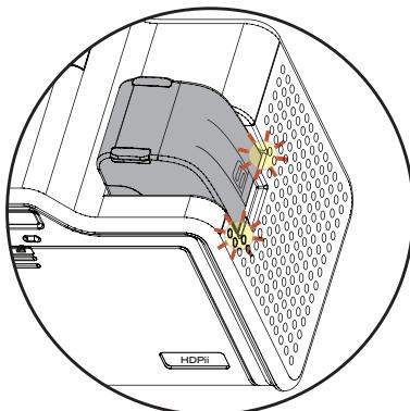
Place card input cartridge onto printer and push until it clicks.
