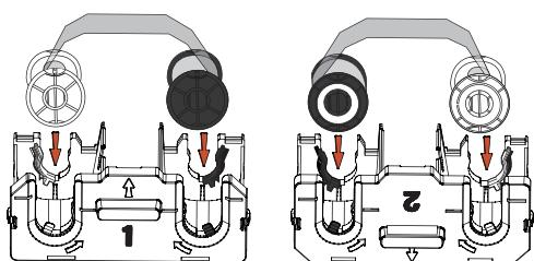
Load lamination rolls into the cartridges until they click.
