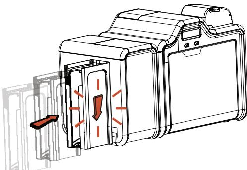
Place card output hopper onto output side (left) of the unit and push down until it clicks.
