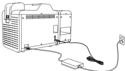
Reconnect power supply and communication cable (USB or Ethernet) to printer.
