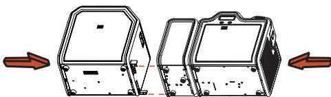
Slide lamination module and printing module together.
