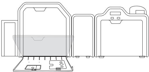
Pull open the Lamination module cover.
