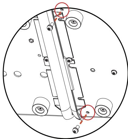
Using the tool and the 2 screws provided, secure the lamination module to the printing module.
