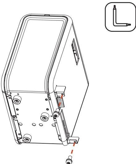
Using the tool provided, remove and save the 2 screws from the bottom of the dual-sided printing module.
