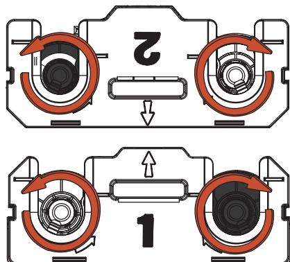
Tighten lamination rolls.
