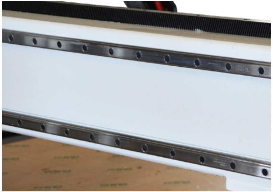
Taiwan Linear Square Guide: 20mm linear square guide with double bearings, an ultra heavy type that achieves a deep grooved raceway with its diameter more approximate to the ball diameter and has high rigidity, vibration and shock resistance, and damping characteristics, which are required for machine tools.
