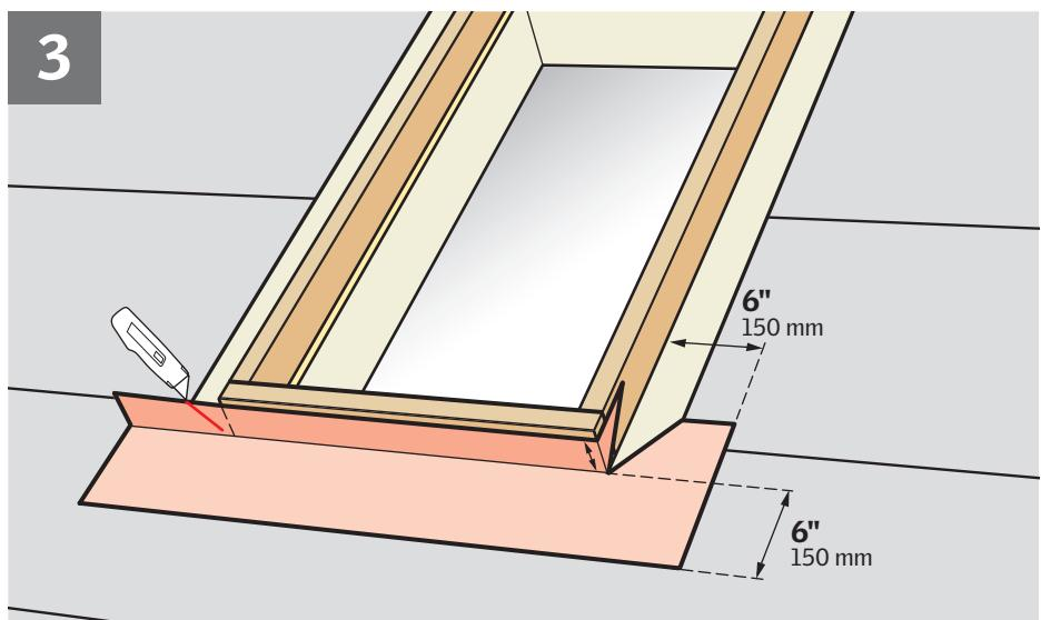
**ENGLISH:** Peel off backing from VELUX adhesive skylight underlayment prior to applying it to roof decking and skylight curb. Ensure that surfaces are clean, dry and free of debris.
