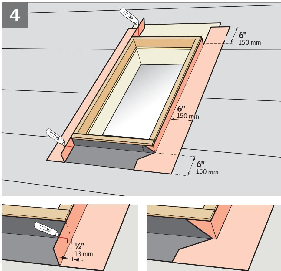
**ENGLISH:** Wrap the sides and the corners of the curb with VELUX adhesive skylight underlayment and create water-shedding laps over roofing underlayment.
