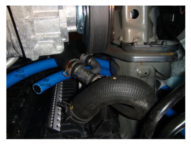
With the I/M hose through the tight spot, attach the check-valve to the I/M hose
