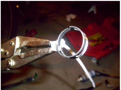
With the factory hose clamp on the new PCV hose, push the new hose onto the factory PCV valve, move the hose clamp till it sits on the end of the hose at the PCV valve, and remove the zip tie locking the clamp in place.
