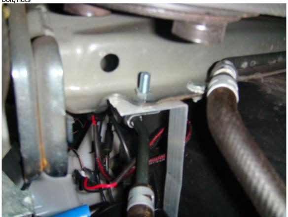
With the OCC mounted, attach the hoses to the OCC with the provided hose clamps. The hose coming from the I/M attaches to the bottom port on the OCC, and the hose coming from the factory PCV mounts to the top port for the Saikou Michi OCCs, the Damond Motorsports OCC ports are opposite. The clamps should be tightened on the OCC, right behind the raised edge on the OCC ports.
