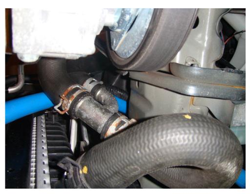
Make sure that the hose is routed in front of the coolant tubes. Now bring the hose over to the factory PCV valve, the pictures should aid as to where it goes after the coolant tubes.
