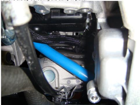
**Step 4:**Begin routing the Intake Manifold hose (blue tape) through the same hose as the new PCV hose. Thy to get it left and underneath of the PCV hose.
