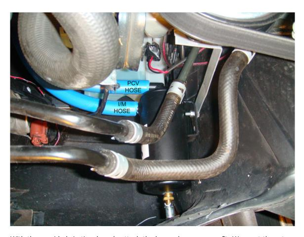
With the provided zip ties, loosely attach the hose where you see fit. We want there to be a little play for the hose to travel as the engine moves, so don't tighten the zip ties all the way, just to secure the hose in place.
