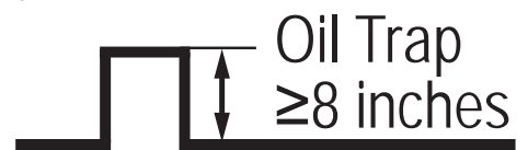
Figure 31: Close Up of An Inverted Oil Trap.
