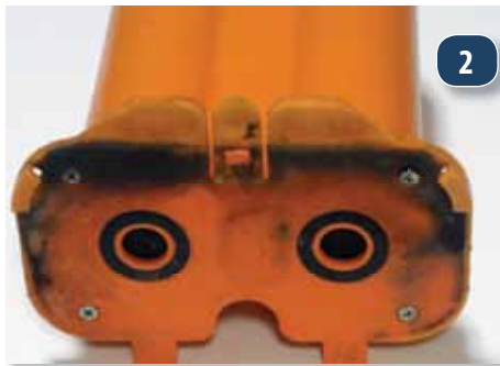
1. After testing, we cut open the homemade tank vent filter; there was no evidence of clogging or contamination of the carbon. There had been some concern that catalytic oxidation of the carbon would lead to sulfur deposits, but there was no sign of this. 2. The Big Orange's slide-out filter unit shows that the gaskets were still good after 30 months of testing. 3. Further disassembly showed that all parts of the Big Orange filter were still in good shape.
