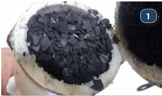
1. After testing, we cut open the homemade tank vent filter; there was no evidence of clogging or contamination of the carbon. There had been some concern that catalytic oxidation of the carbon would lead to sulfur deposits, but there was no sign of this. 2. The Big Orange's slide-out filter unit shows that the gaskets were still good after 30 months of testing. 3. Further disassembly showed that all parts of the Big Orange filter were still in good shape.
