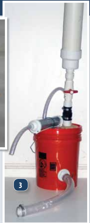
1. Testers used a 1-pound ball-peen hammer to weight down the hoses during the hose-flexibility test. 2. We installed a homemade, PVC vent filter on the PDQ test boat. 3. Five-gallon buckets with tight lids were fitted with sanitation hoses and tank vent filters to create mini holding tanks for this test.
