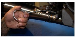
20. Mount muffler to bracket using supplied 8mm screw, washer and nut
