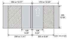
Maximum Cover Sheet Fore-edge Length: 660 mm / 25.98° (Up to 350 mm / 13.77° towards from the clamp face, and up to 310 mm / 12.20° backwards from the clamp face.) Additional two scoring lines for flap cover can be made in
