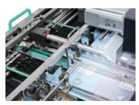
■ The hold-down roller sets to the proper position to prevent the sheet from bouncing back after hitting the knife stopper. The roller position is automatically adjusted when the sheet or fold pattern is changed.
