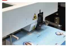
Quality polyurethane rotor provides high speed feeding without scratching. The suction angle adjustment enables stable feeding by adjusting the angle of suction air according to the sheet condition. The supersonic and photoelectronic double feed detect sensors come standard for superior double feed protection.
