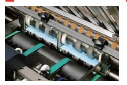
Perforation, slit perforation, scoring and slitting can be performed. Durable scoring unit is employed for accurate scoring. Optional devices are available for strip trimming of multiple-up jobs, trimming the closed side of glued signatures and punch perforation.
