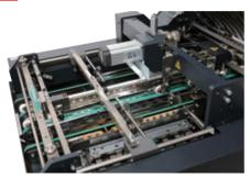
Newly designed rigid and durable knife unit provides consistent quality knife folding. No need to open the knife cover for setup. The entire setup, such as installing the stopper guide, knife angle adjustment and hold down roller position is automated.
