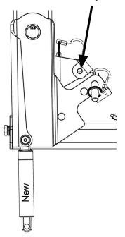
4. Rotate damper, reinstall bolt/bushing and lanyards
