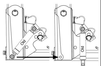
2. Install damper with existing bolt/bushings
