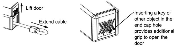
Insert each cable through bikes (or front tires) and lock the cables together or to the rack. Cable doors can be closed with cable extended.
