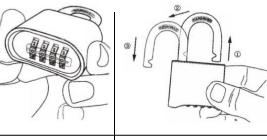
2. Pull the shackle out and rotate it 180 degrees and push it in toward the lock and hold it in.
