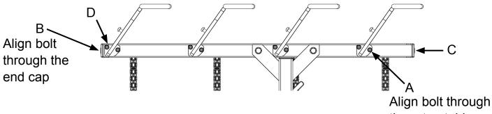
Install End Caps at location B and C (sliding door at top)
