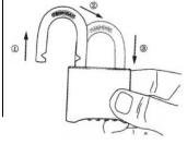
4. Rotate back. Always leave it locked so the combination can't be changed.
