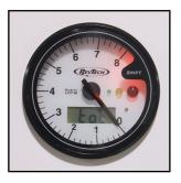
Next step round the setup menu is the odometer function. This is where your tach counts up and retains the total mileage your motorcycle has covered since the unit was installed. If your display says **tot** like the picture on the left, you're there.
