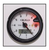
Next item on the setup menu is the Filter. This is to do with configuring the tach to respond to the signal it receives. Normally this is set to **Fon** (filter on) meaning the tach tends to reject unwanted signals. CDI type ignitions tend to have very short ignition pulses and you may have to set this option to **Foff** for the tach to "see" the signal.
