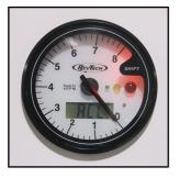
From **SSP**, tap the button once to get to **FSP**. As you would expect, **FSP** is the finish speed for the acceleration timer. Set it in exactly the same way as the start speed: hold down the button to get into the routine, tap the button until you get the number you want, leave the button for 4 seconds to exit.
