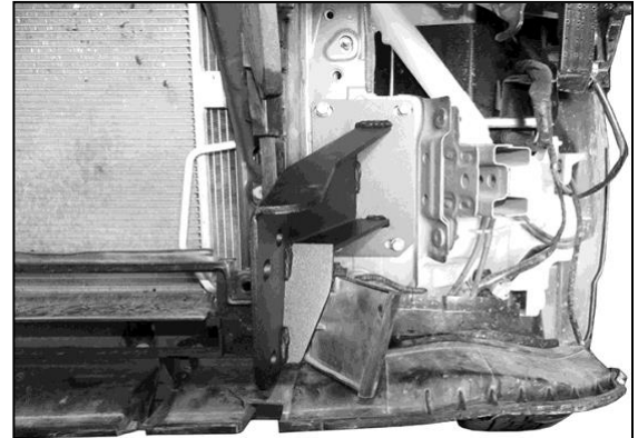
(Fig 6) Driver/left Bumper Bracket installed
