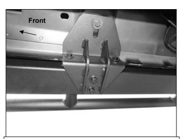
(Fig 15) Rocker Guard attached to #2 Center Bracket
