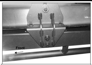
(Fig 14) Rocker Guard attached to #3 Center Bracket
