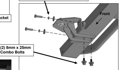
(Fig 16) Attach Rocker Guard to front Bracket
