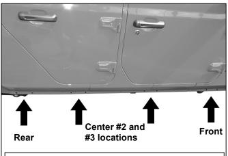
(Fig 1) Passenger/right side mounting locations. Use a 5/16" drill bit to open mounting holes in pinch weld only if necessary.
