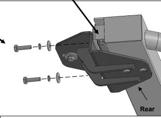
(Fig 10) Slide Rocker Guard in against pinch weld. Attach Rocker Guard to rear Bracket, pinch weld and Double Nut Plate. Leave hardware loose
