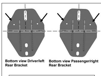
(Fig 7) Rear Brackets look similar to Center Brackets but are slightly angled. NOTE: Brackets also feature small holes in plate for ID purposes, (arrows).
