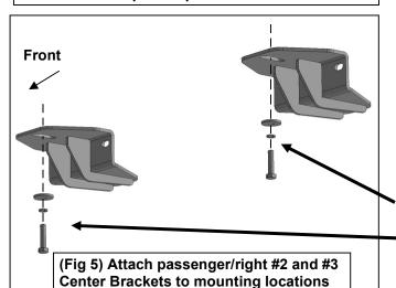
8mm x 35mm Hex Bolt 8mm Lock Washer 8mm x 28mm Large Flat Washer
