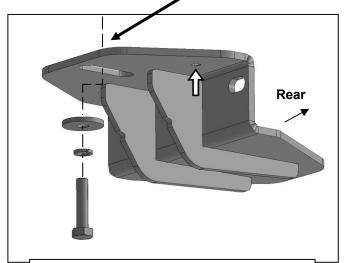
(Fig 8) Attach passenger/right Rear Bracket NOTE: Brackets feature small holes in plate (arrow) for ID purposes only (Fig 7).
