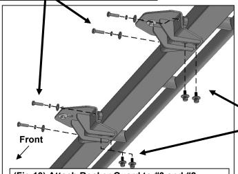
(Fig 13) Attach Rocker Guard to #3 and #2 Center Brackets. Do not tighten hardware at this
