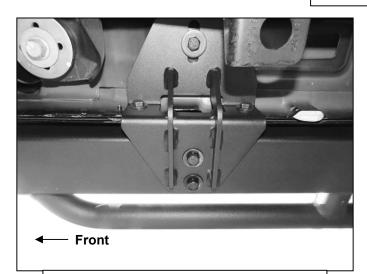
(Fig 17) Level and adjust Rocker Guard and fully tighten all hardware.
