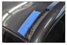
STEP 10 - Place rubber gasket in gutter.
