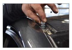
STEP 8 - Insert supplied Grip-Sert into the holes. (Small amount of silicone on splined area is recommended)
