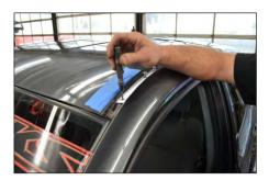
STEP 6 - Mark front hole with center punch. Double cab trucks use factory rear Nut-Certs already installed. Access cab trucks will require marking the rear hole and will not use the center hole.
