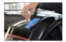
STEP 1 - Tape off truck to protect paint from scratches. Lift up rain gutter molding in front corner.
