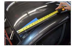
STEP 3 - From the front windshield edge of molding, measure out 2.5" and 10.75" and make a mark.
