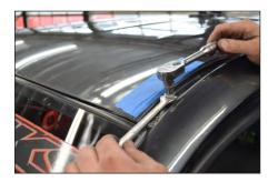
STEP 9 - Use tool to fasten Grip-Sert by tightening down the bolt while placing wrench on center nuts. DO NOT let Grip-Sert turn when tightening.
