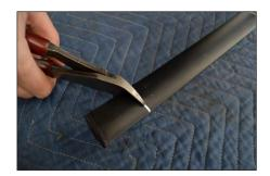
STEP 4 - Cut rubber molding on marks and remove center. Reinstall front and rear molding pieces.
