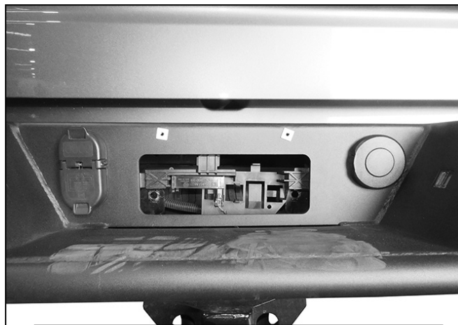
(Fig 28) Trailer plug, spare tire lock, license plate plugs and TPMS antenna installed
