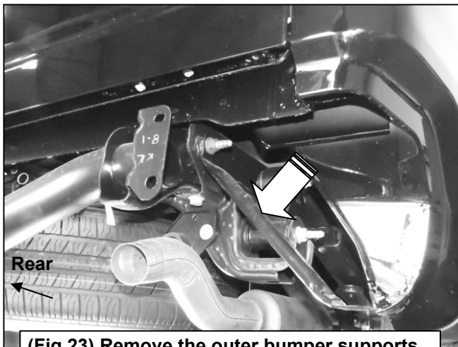
(Fig 23) Remove the outer bumper supports from both sides of the frame (arrow)
