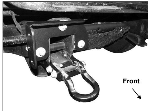
(Fig 9) Attach Tow Hook to Extension Bracket
