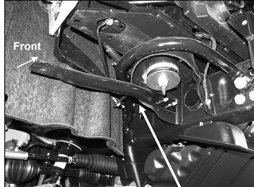
(Fig 4) Remove outer bumper support brackets
