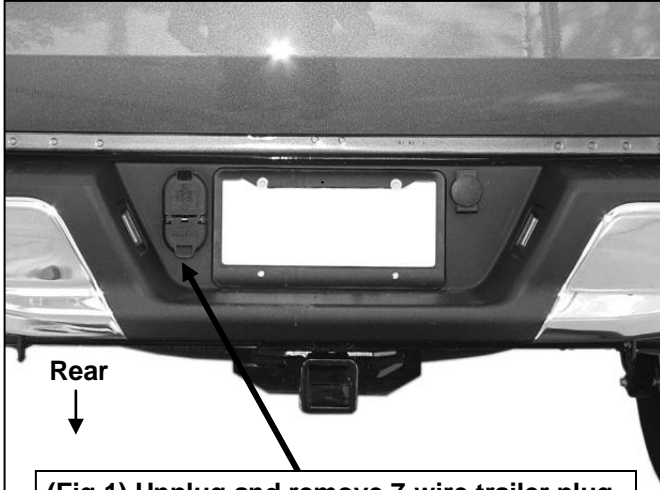
(Fig 1) Unplug and remove 7-wire trailer plug
