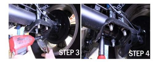
5. Use the floor jack to lift the rear axle, keeping the pin aligned with either the centered hole or the offset hole, and install the new u-bolts with the provided hardware. **NOTE: TORQUE U-BOLTS TO 100 FT/LBS**
