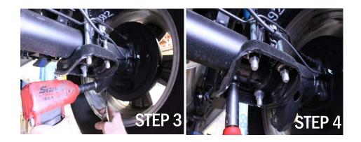
3. Use the floor jack to lift the rear axle, keeping the pin aligned with either the centered hole and install the new u-bolts with the provided hardware. **NOTE: TORQUE U-BOLTS TO 100 FT/LBS**
