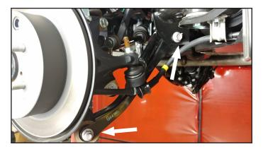
**30. Loosen but do not remove the rear lower control** arm bolt at the subframe.
