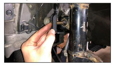
**18. Install the 1/4" thick spacer washer onto the end** of the sway bar link.
