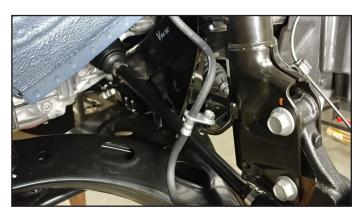
15. The cam bolt's head flange has hash marks that correspond to a notch on the strut body. Rotate the cam bolt until the hashes are facing the inside of the vehicle, and align the last hash mark with the notch. This will set camber to maximum negative. Torque both bolts to 95 ft-lbs.
