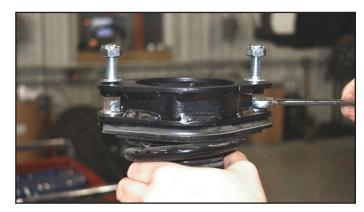
**34.** Install the completed strut assembly to the car using the provided M10 flange nuts. Do not tighten at this time. A helper is recommended.
