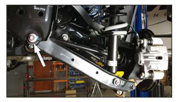
31. Support the strut and lower control arm, remove the lower strut and knuckle bolts. Lower the control arm down, while holding the strut. Remove the strut from the vehicle. A helper is recommended to hold the strut from falling.
