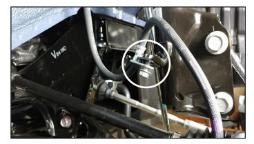
**7. Disconnect the ABS wiring harness clip from the** strut body and let hang out of the way.
