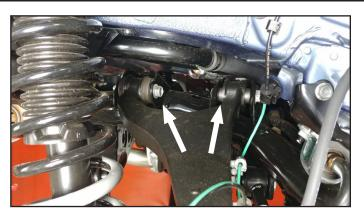
**29. Loosen but do not remove the front lower control** arm bolts.
