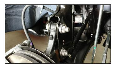
9. With the lower control arm supported by the jack stand, release the knuckle from the strut body and let it, along with the lower control arm, hang out of the way. Be careful not to over-extend the CV axle, brake line or ABS harness (adjust the jack if necessary).
