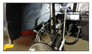
10. Remove the three (3) nuts that attach the upper end of the strut to the strut tower (accessed from the engine bay, as the hood should already be propped open). Do not let the strut fall as you remove the last bolt. It may be helpful to have a friend hold up strut as the bolts are removed. Carefully lower the strut and remove it from the vehicle.
