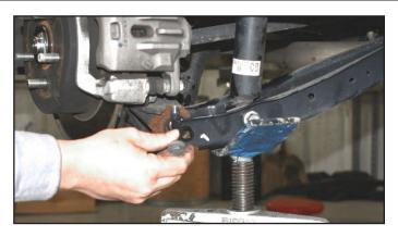
ing headlight feature, there is a small linkage attached to the driver's side rear lower control arm. The Body Armor 4X4 kit comes with an Headlight Auto-Aim Linkage Bracket to restore the headlight load-leveling feature. Disconnect the stock linkage from the lower control arm, install the bracket, and reconnect the linkage to the bracket.
