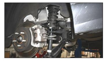
35. Raise the lower control arm into place and install the lower strut hardware. Do not tighten at this time. Use the jack and raise the lower control arm up to set pre load on the strut. Re-install the lower knuckle bolt. Torque to 95 ft-lbs.
