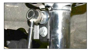
**20.** Repeat the previous steps to install the other strut spacer on the opposite side of the vehicle. Once both ends of the sway bar have been re-attached, torque the sway bar end links and brackets to 45 ft-lbs.
