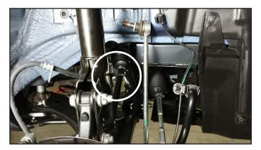
8. Remove the two large bolts that attach the strut to the steering knuckle. Note the orientation and position of the bolts, as they will need to be re-installed in the same configuration. The bolts are specific to upper and lower mounting locations and direction of install (the upper one is a cam bolt).
