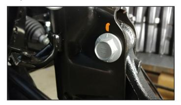
16. Re-install the brake line bracket to the strut body, but with the bracket rotated as shown in the photo. Originally the brake line was attached from the bottom upwards to the strut, now it will be mounted to the top of the strut body using the factory hardware.
