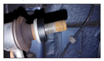
**19. Attach the sway bar end link to the newly-in-**stalled bracket using the factory hardware.
