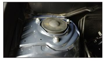
**11.Install the strut extension onto the removed** strut assembly using the factory nuts and 14mm
